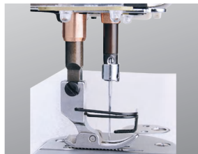
针杆表面DLC钻石样涂层处理(选购) DLC disposal needle bar(optional)
